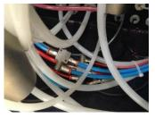
Make reference to the pneumatic scheme "**Ps**" for cabling the pneumatic plant. Cut the existing red and blue 6mm size air tubes in the bottom of the saw. These pipes already control the cylinders of the vertical clamp.
