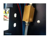
Have the 8mm size hole done in both left and right corner side for fixing the horizontal clamp support.
