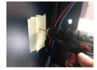
Drill the hole where the paper has been marked from the inside of the body.
