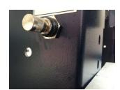
Drill the same hole from the outside and make an 8mm diameter size.
