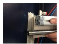
Place the horizontal clamp on top of the working bench and insert it in the internal corner of the saw having the two thread holes matching with the fixing frontal holes of the carpentry.
